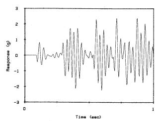
Fig. 3 Acceleration response of the sailplane (case A).
