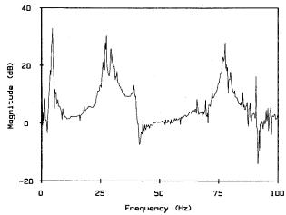
Fig. 8 Frequency-response function from frequency-domain techniques.
