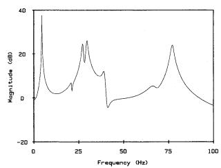
Fig. 7 Frequency-response magnitude plot of the reduced model.
