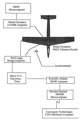
Fig. 1 Schematic of experiment.
