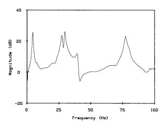
Fig. 9 Averaged frequency-response function from frequency-domain techniques.
