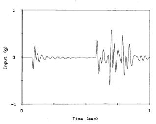
Fig. 4 Input to the sailplane (case B).
